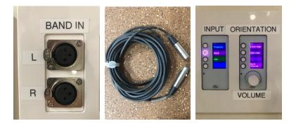
To control the sound level, first be sure the output level of your source device is turned up to at least 75%, then be sure the **INPUT** control is switched to **Band** (middle button, purple background), and adjust the volume knob as desired.
