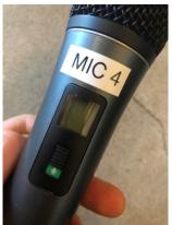
The base of the microphone unscrews in case the two AA batteries need to be replaced.
