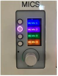
Then on the **MICS** control, select the number of any mic you want to set a level for, and use the volume knob at the bottom to get a sound check. These levels can be adjusted at any time during a presentation. You simply need to remember who is holding which numbered mic.
